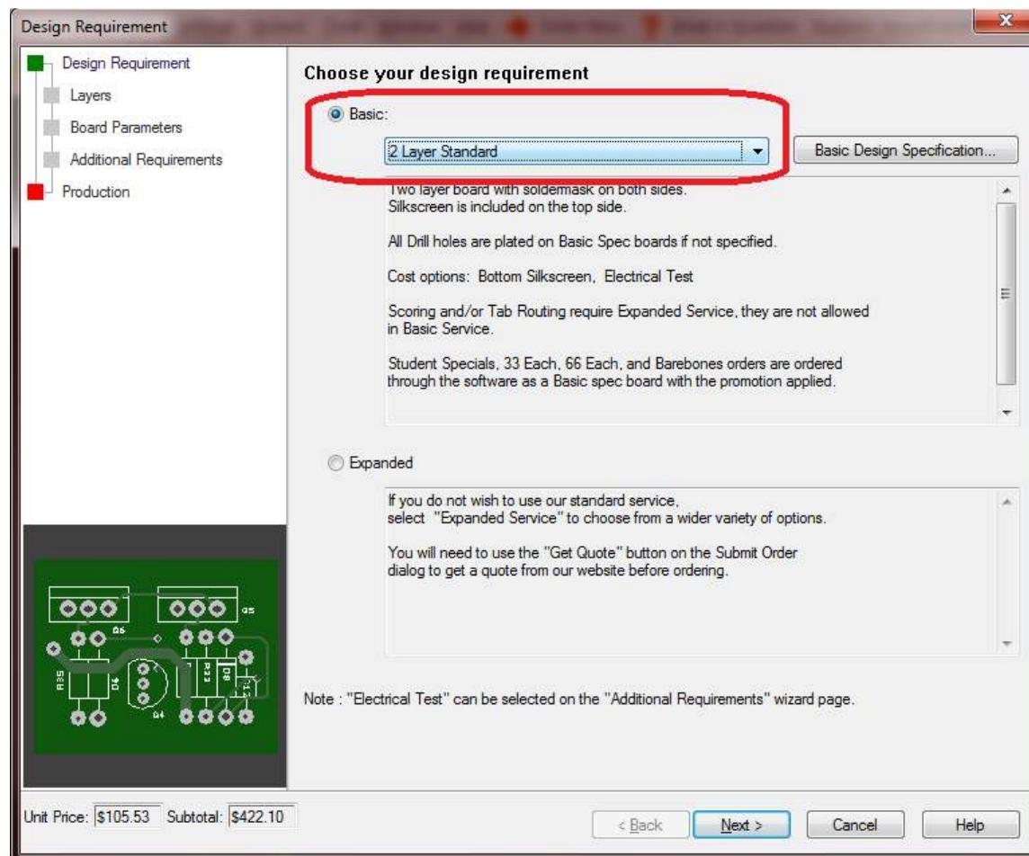
The PCB Configuration is also where one can set up the board order. Make sure your order matches the Barebones order specs found here: <https://www.4pcb.com/pcb-prototype-2-4-layer-boards-specials.html>
