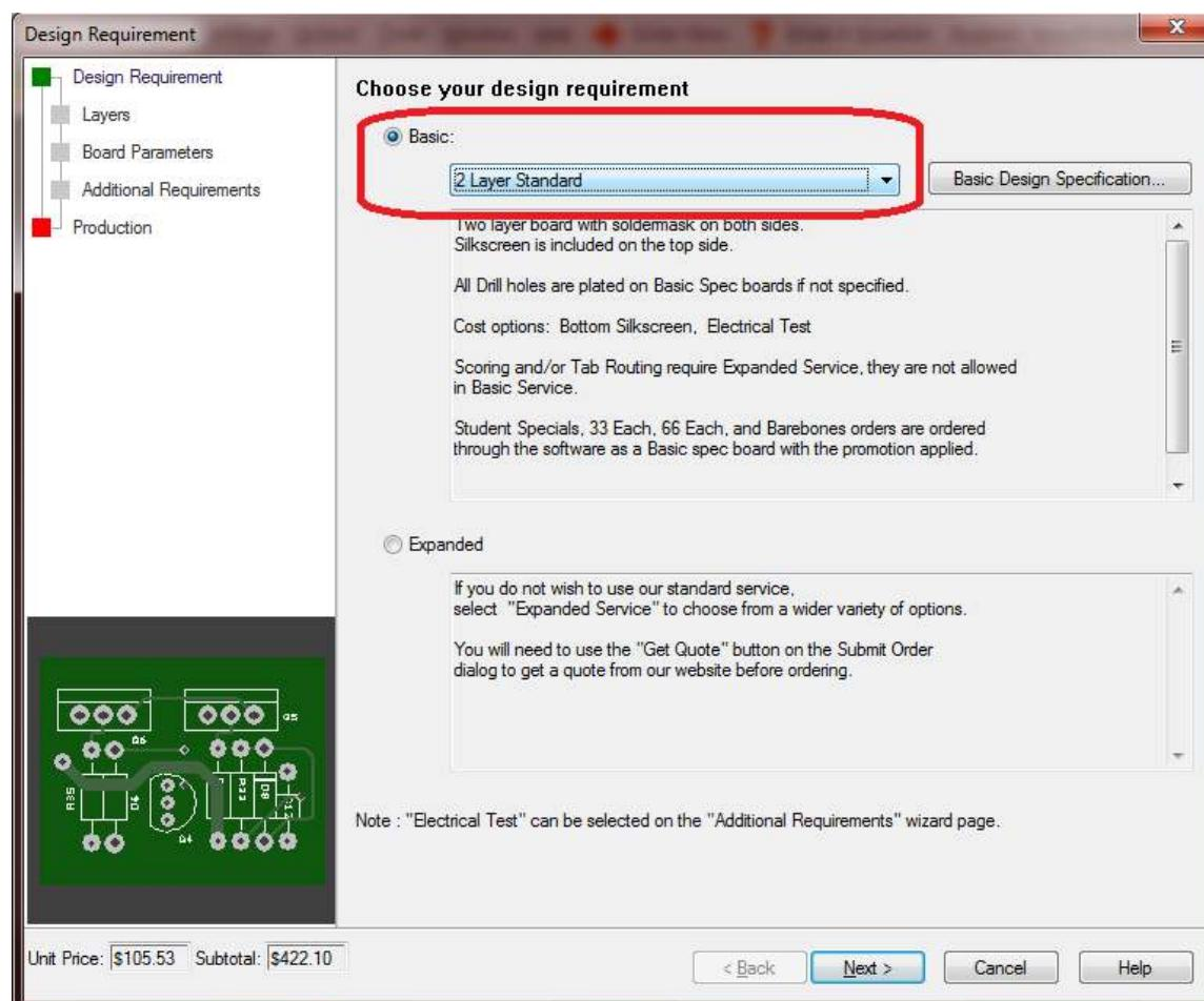
The PCB Configuration is also where one can set up the board order. Make sure your order matches the 33 special or 66 special specs found here: <https://www.4pcb.com/pcb-prototype-2-4-layer-boards-specials.html>
