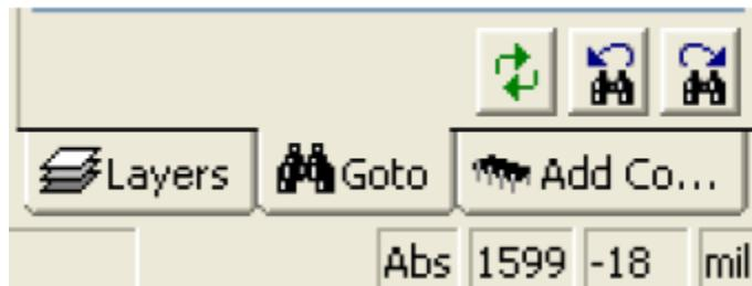
The Status Bar is in the lower right frame of the application and displays current settings such as the units setting, the current coordinates of the cursor, etc. When an item is selected (such as a pad), a list of information about that item is displayed in the Status Bar, such as the pad style, the net of the pad, the layer it exists on.
