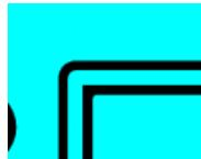
**Dark Cyan/Teal:** Bottom copper with soldermask clearance. In the properties drop down, this will show as [Bottom].
